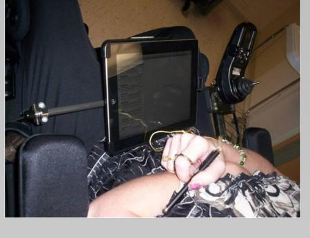
ITERATIVE DESIGN #1: Use of touch accommodations to compensate for progressive motor access limitations even with stylus to allow for longer dwell times and minimize inadvertent selections during typing Speech-recognition access not feasible d/t dysarthria severity.
