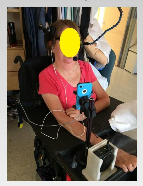
ITERATIVE DESIGN #3: Add Amazon Echo Dot for speech-recognition input paired with Logitech Harmony Hub for IR signal blast to TV. Field microphone on Echo Dot more sensitive than that on iPhone, with the result that no external microphone required for access.
