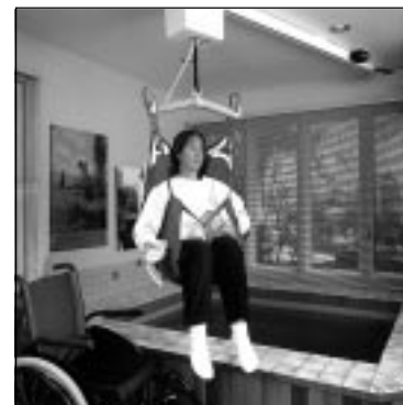
Overhead Lift: Residents are safely transported with the Waverly Glen transactive. The sling allows residents to be lifted in a sitting position, saving time because it requires less maneuvering.
